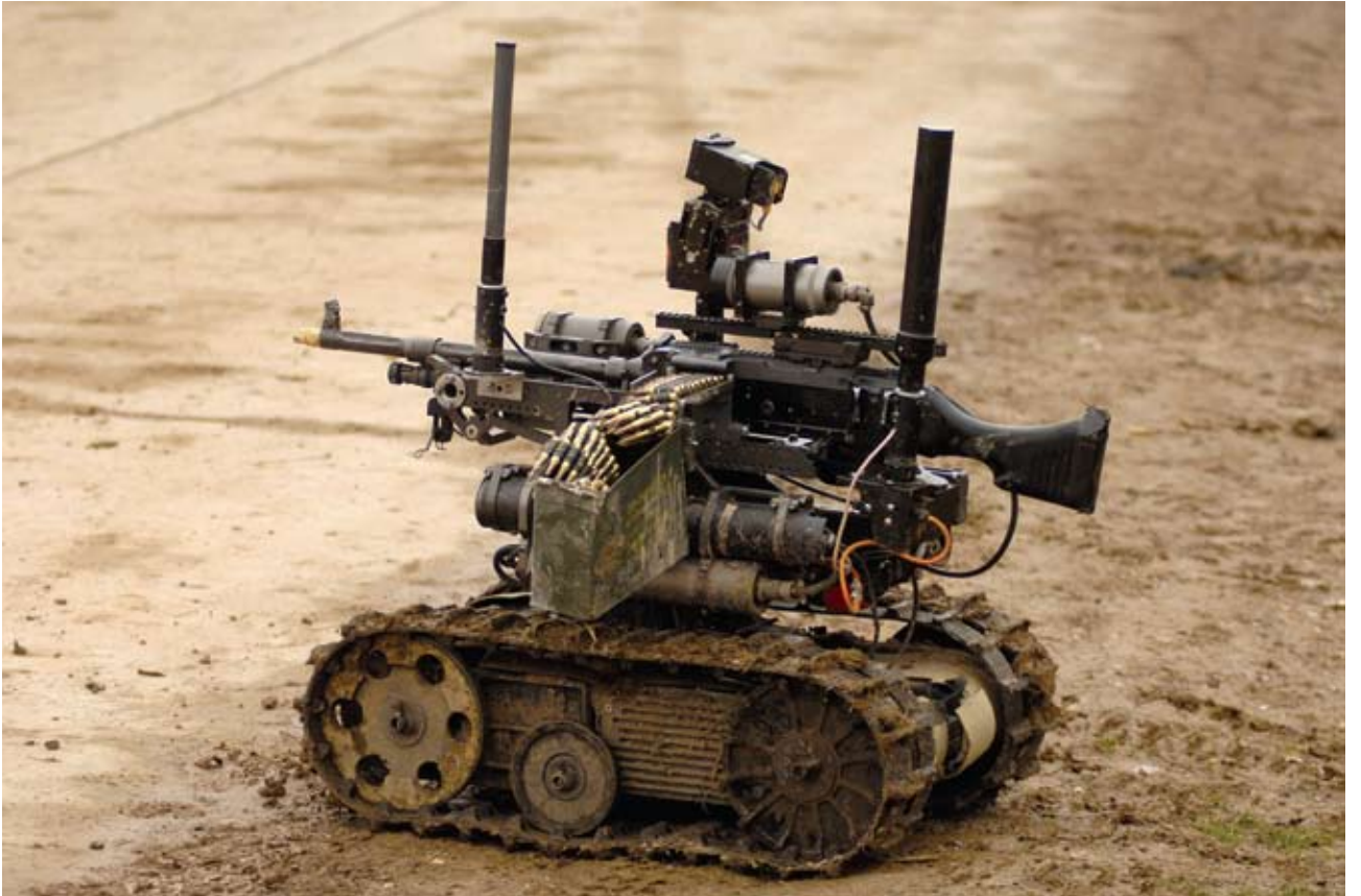
Prototype bewapende SWORDS. © UK MOD Crown Copyright
