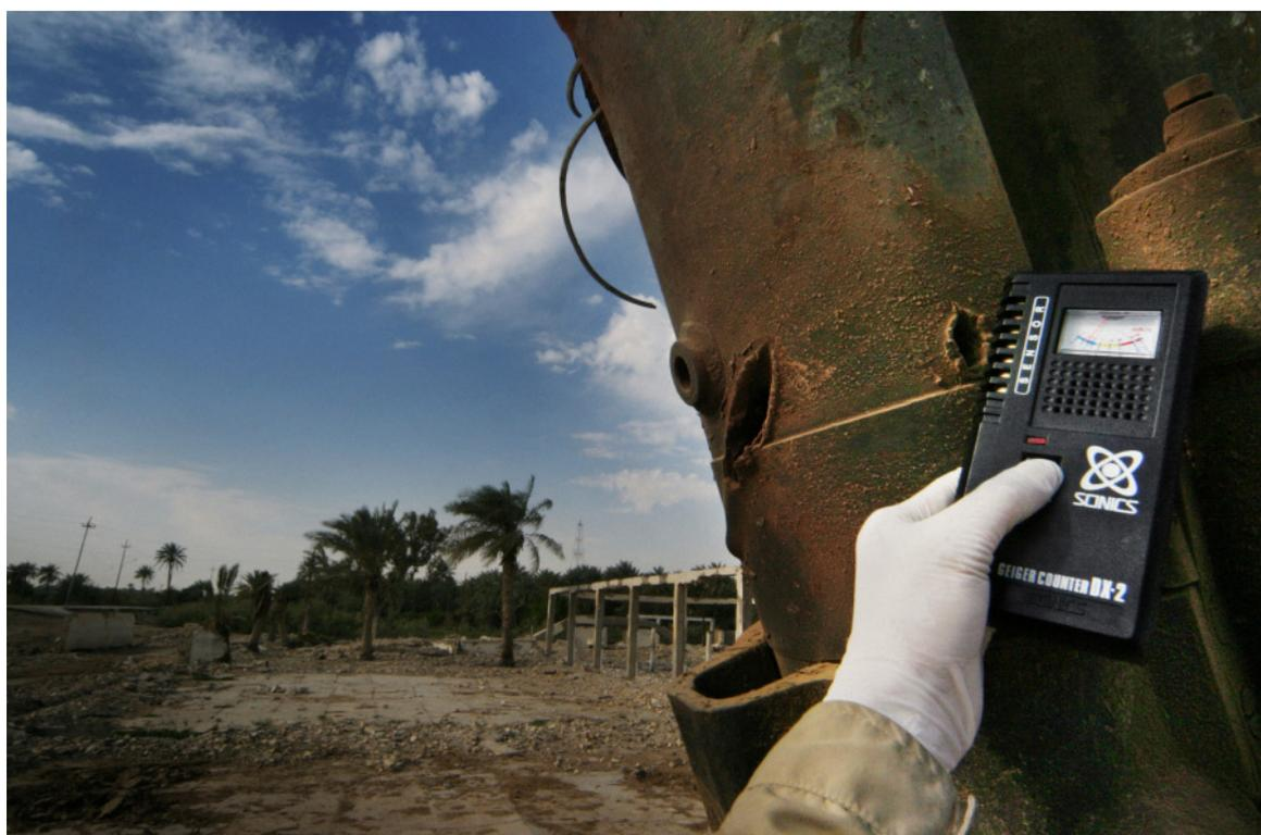
**Scars from a DU strike on an Iraqi tank displaying high levels of residual radioactivity**
